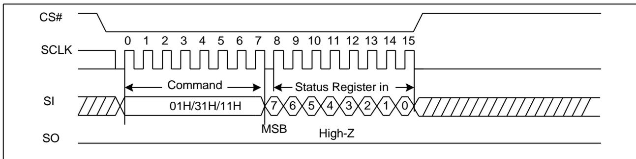
**Figure7a. Write Status Register Sequence Diagram (QPI)**
