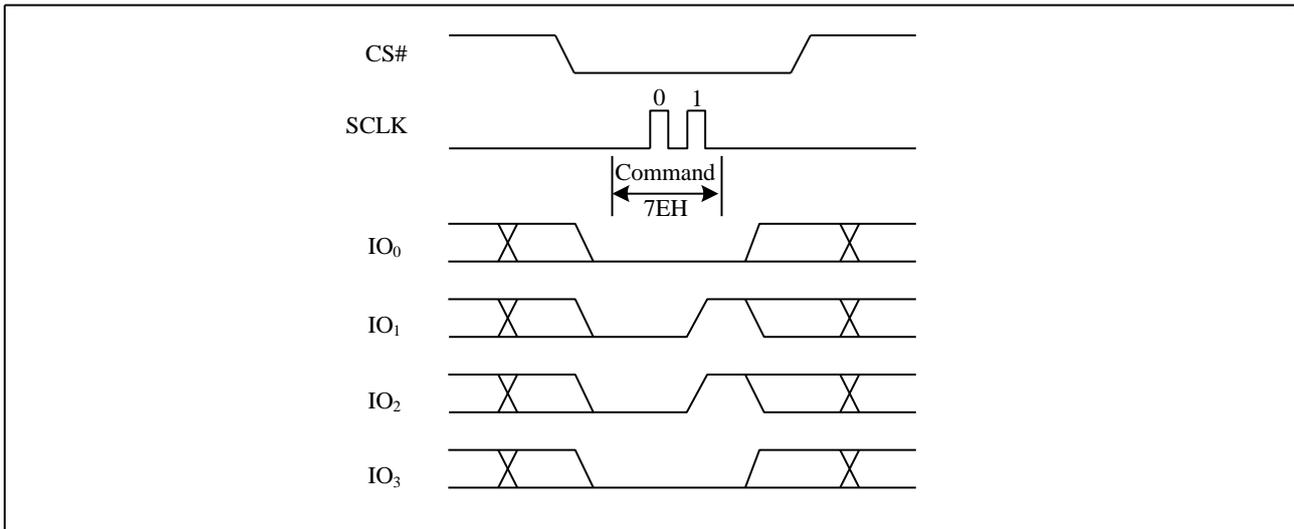
**Figure38. The Global Block/Sector Unlock Sequence Diagram**
