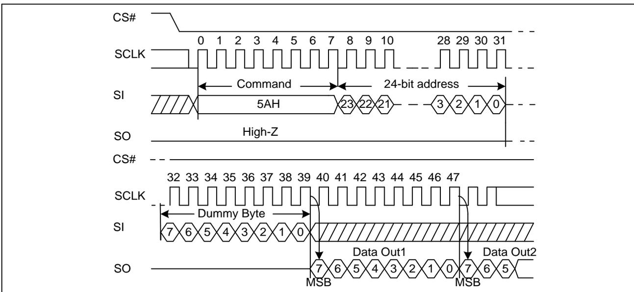
**Figure45a. Read Serial Flash Discoverable Parameter command Sequence Diagram (QPI)**
