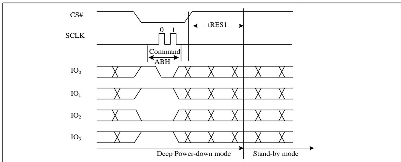
Figure24. Release Power-Down/Read Device ID Sequence Diagram
