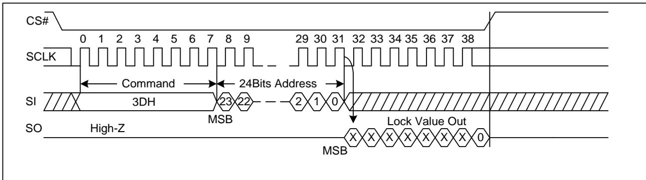
**Figure36a. Read Individual Block/Sector lock command Sequence Diagram (QPI)**
