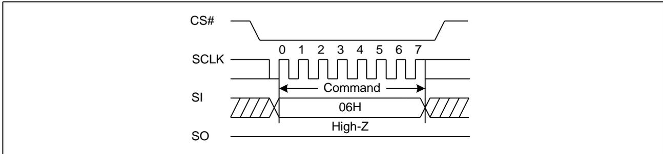
**Figure3a. Write Enable Sequence Diagram (QPI)**
