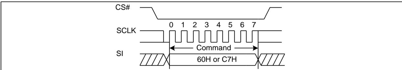
**Figure21a. Chip Erase Sequence Diagram (QPI)**
