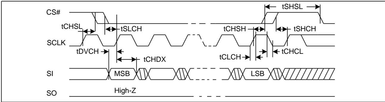
**Figure50. Output Timing**
