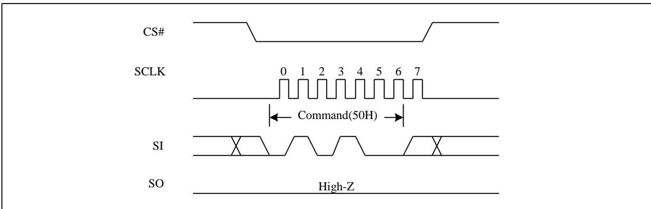
**Figure5a. Write Enable for Volatile Status Register Sequence Diagram (QPI)**
