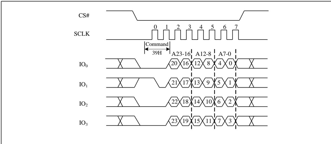
Figure36. Read Individual Block/Sector lock command Sequence Diagram
