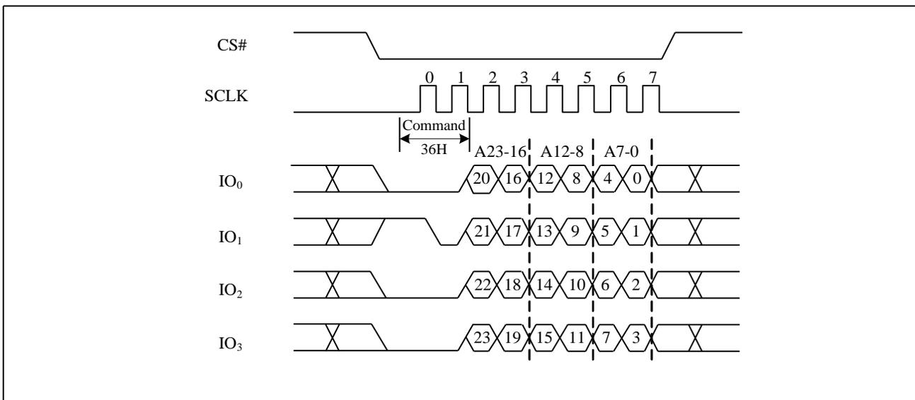
Figure35. Individual Block/Sector Unlock command Sequence Diagram
