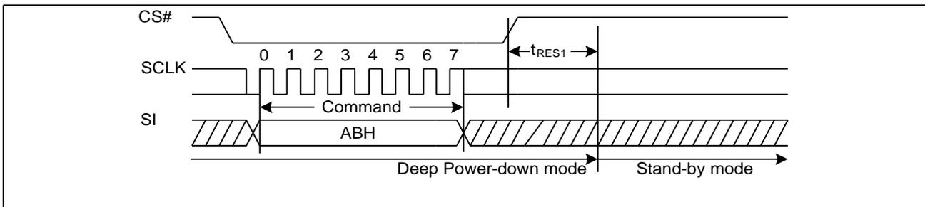
**Figure23a. Release Power-Down Sequence Diagram (QPI)**
