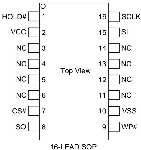
Note: Only for special order, Pin 3 is RESET# pin. Please contact GigaDevice for detail.
