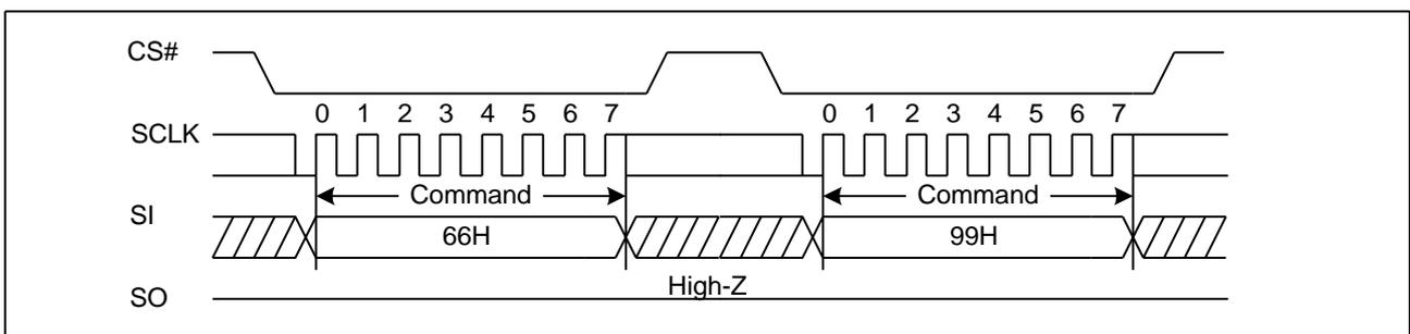
**Figure44. Enable Reset and Reset command Sequence Diagram (QPI)**
